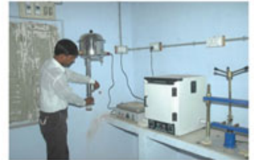
Distilled Water Plant
